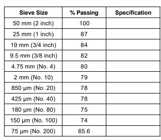
**Test Method:** Method A (Composite Sieving)
