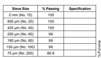
**Test Method:** Method A (Composite Sieving)
