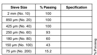
Test Method: Method A (Composite Sieving)
