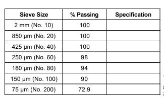
**Test Method:** Method A (Composite Sieving)
