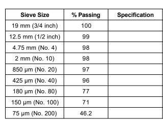
Test Method: Method A (Composite Sieving)
