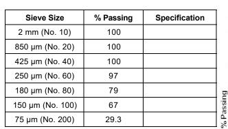
**Test Method:** Method A (Composite Sieving)
