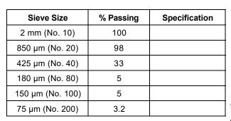
Test Method: Method A (Composite Sieving)
