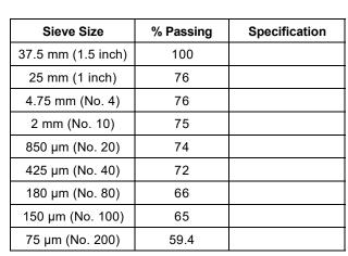
Test Method: Method A (Composite Sieving)
