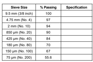
**Test Method:** Method A (Composite Sieving)
