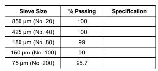
Test Method: Method A (Composite Sieving)
