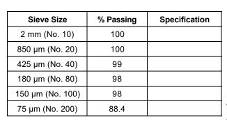
Test Method: Method A (Composite Sieving)
