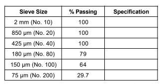
**Test Method:** Method A (Composite Sieving)
