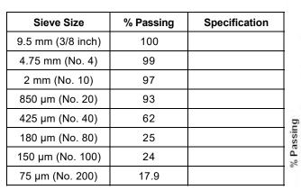
**Test Method:** Method A (Composite Sieving)
