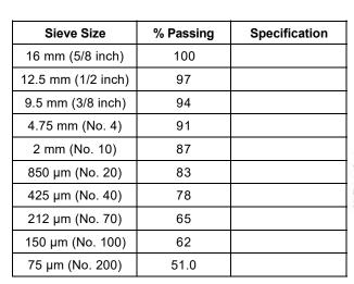
**Test Method:** Method A (Composite Sieving)
