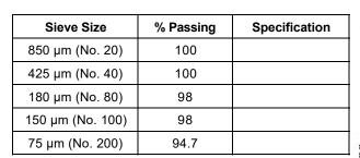
**Test Method:** Method A (Composite Sieving)
