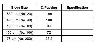
Test Method: Method A (Composite Sieving)
