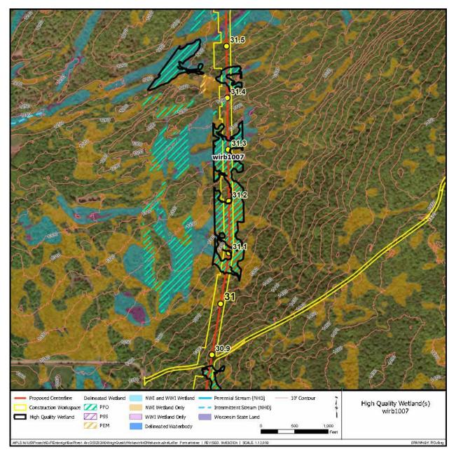
Enbridge has completed a desktop analysis of an alternative route that would avoid/minimize impacts to this wetland. The alternative would place the pipeline route east of and upslope of the wetland. Based on desktop data, the alternative would cross fewer wetland resources, but would place the line on steeper topography and side-slope areas. While the route may be technically feasible based on a desktop review, no field constructability analysis has been
