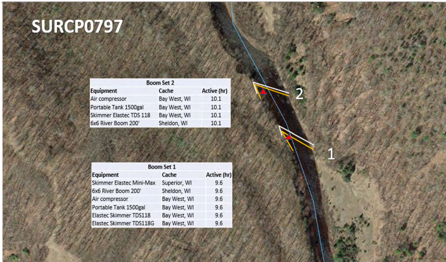
Figure 3-21. Response layout for MCP SURCP0797 on the Bad River. Red triangles are skimmer placement locations, orange lines represent containment boom, and white lines represent sorbent boom. The sorbent boom was not simulated in the model.
