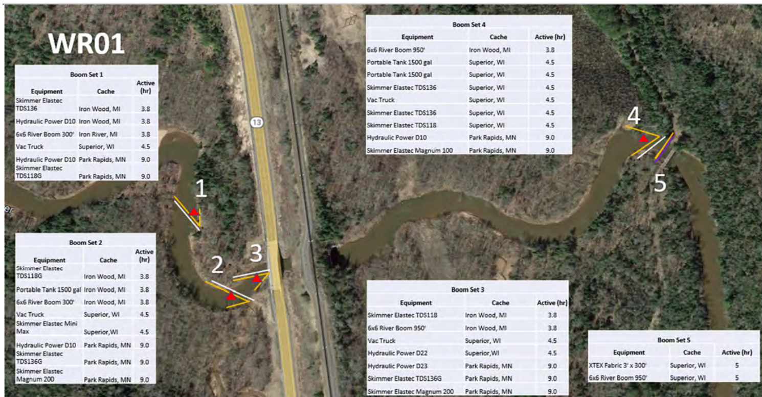
Figure 3-25. Response layout for MCP WR01 on the White River. Red triangles are skimmer placement locations, orange lines represent containment boom, white lines represent sorbent boom, and the purple line represents X-Tex fabric. The sorbent boom and X-Tex fabric were not simulated in the model.
