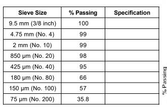
**Test Method:** Method A (Composite Sieving)
