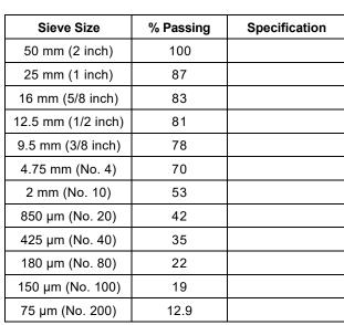
**Test Method:** Method A (Composite Sieving)
