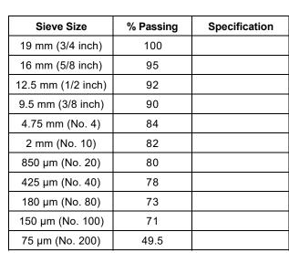
**Test Method:** Method A (Composite Sieving)
