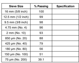
**Test Method:** Method A (Composite Sieving)
