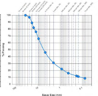
**Test Method:** Method A (Composite Sieving)
