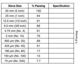
**Test Method:** Method A (Composite Sieving)
