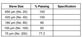
**Test Method:** Method A (Composite Sieving)
