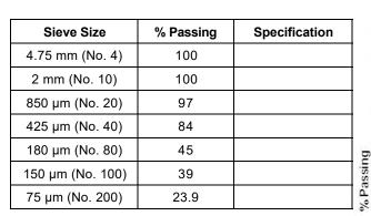
**Test Method:** Method A (Composite Sieving)
