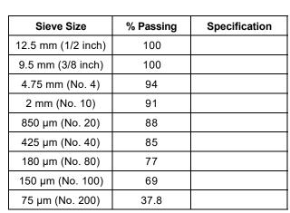
**Test Method:** Method A (Composite Sieving)
