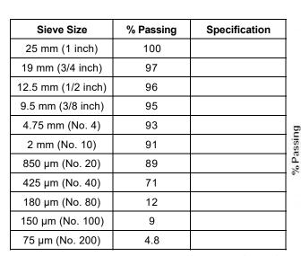
**Test Method:** Method A (Composite Sieving)
