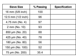
**Test Method:** Method A (Composite Sieving)
